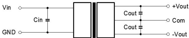
Figure 1. Typical external circuit
