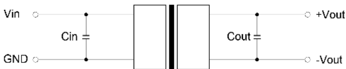
Figure 1. Typical external circuit
