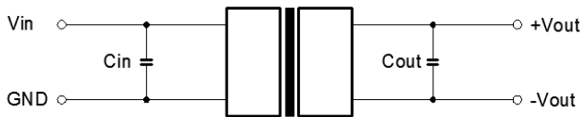
Figure 1. Typical external circuit
