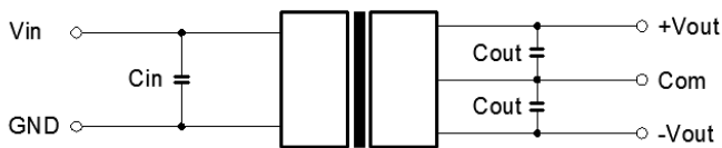
Figure 1. Typical external circuit
