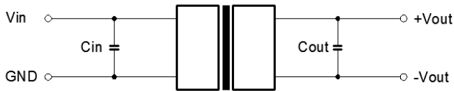
Figure 1. Typical external circuit
